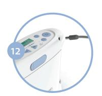
Connect the AC power supply cord to the Inogen One® G<sub>3</sub> and plug the power supply AC cord into an electrical outlet. **Do Not Power ON the Inogen One® G<sub>3</sub> concentrator.**
