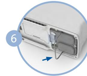
While holding the button open, slide the column assembly out of the device by pulling on the column pull handle.
