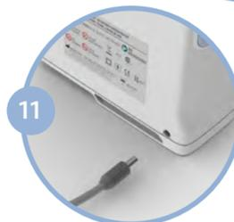
Connect the AC power supply cord to the Inogen One<sup>®</sup> G4 and plug the power supply AC cord into an electrical outlet. Do Not Power on the Inogen One<sup>®</sup> G4 concentrator.
