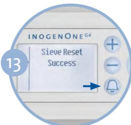
Press the alert/bell button once and screen will display "sieve reset success." Press the power button to turn on the Inogen One<sup>®</sup> G4, and use normally.
