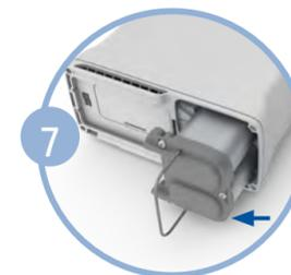
Remove the columns completely from the Inogen One<sup>®</sup> G4. Both columns are removed as one piece.
