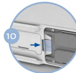
Push the column assembly into the device such that the columns are fully seated into the Inogen One<sup>®</sup> G4 concentrator. The spring loaded latch button should fully return to the closed position.
