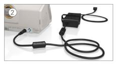
Plug the power connector into the rear of the device. Connect one end of the power cord into the power supply unit and the other end into the power outlet.
